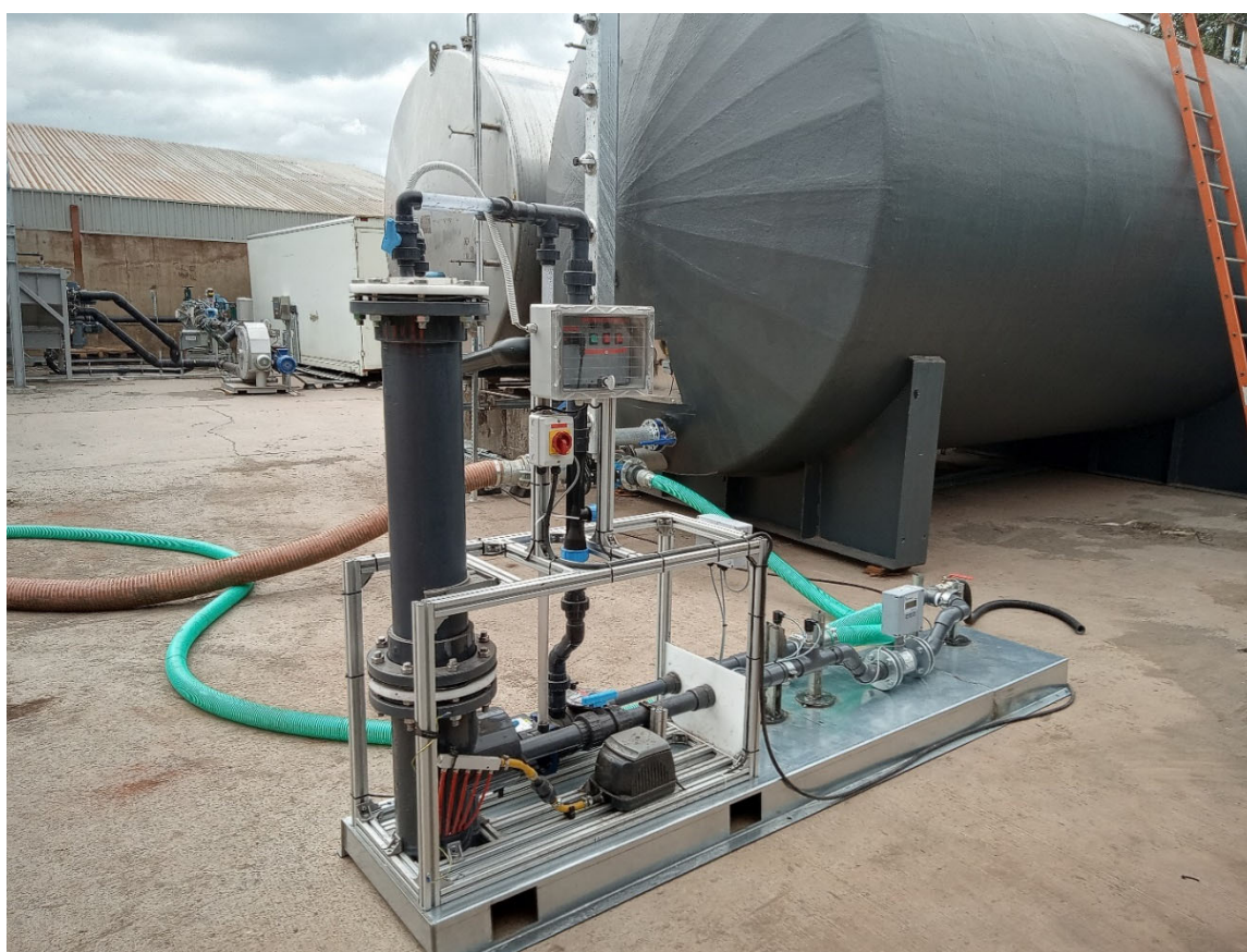
Figure 2. Photograph of NB-generation unit. The vertical cylinder is the electrostriction chamber.
