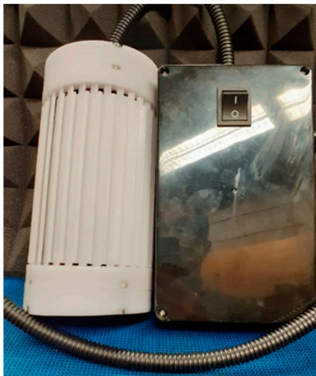
Figure 6. Prototype submersible NB generator used for laboratory-based ML model development.
